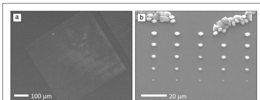
**Figure 3.** Scanning electron microscopy images of the microdot array made from PEGDA/Cultrex hybrid material: (a) A 500  $\mu\text{m}$  by 500  $\mu\text{m}$  microdot array with a dot diameter of 2  $\mu\text{m}$  and a pitch of 20  $\mu\text{m}$ ; (b) dose test of microdot fabrication, the laser exposure time decreased from the top row to the bottom row.
