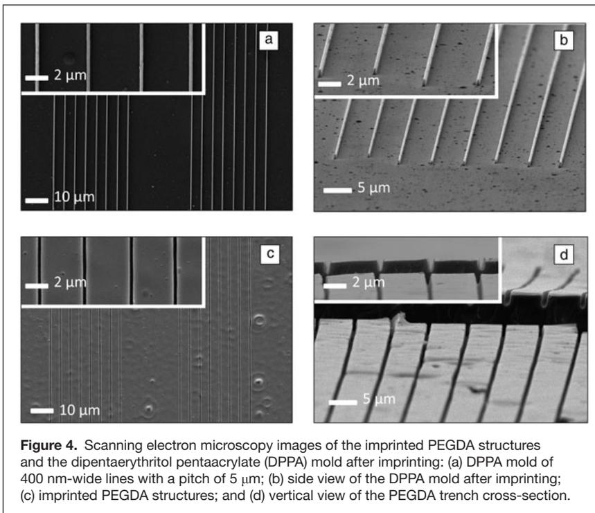
**Figure 4.** Scanning electron microscopy images of the imprinted PEGDA structures and the dipentaerythritol pentaacrylate (DPPA) mold after imprinting: (a) DPPA mold of 400 nm-wide lines with a pitch of 5  $\mu\text{m}$ ; (b) side view of the DPPA mold after imprinting; (c) imprinted PEGDA structures; and (d) vertical view of the PEGDA trench cross-section.
