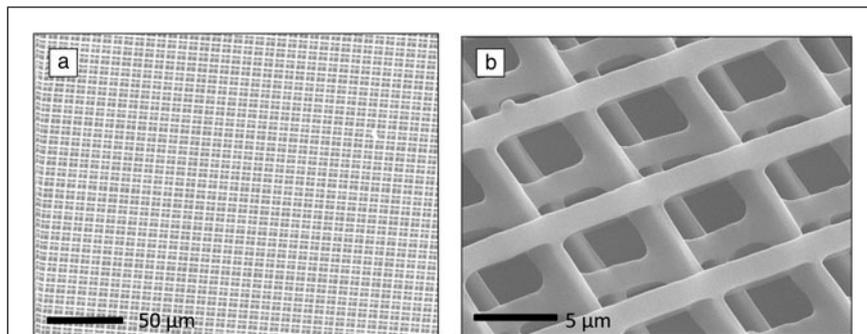
**Figure 2.** Scanning electron microscopy images of the three-dimensional PEGDA scaffold: (a) Six-layer woodpile scaffold of 1  $\mu\text{m}$ -wide lines with a pitch of 8  $\mu\text{m}$ ; (b) magnified view of the scaffolds. The distance between adjacent layers is 3  $\mu\text{m}$ .
