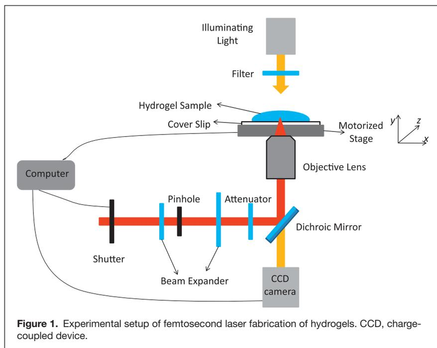
**Figure 1.** Experimental setup of femtosecond laser fabrication of hydrogels. CCD, charge-coupled device.
