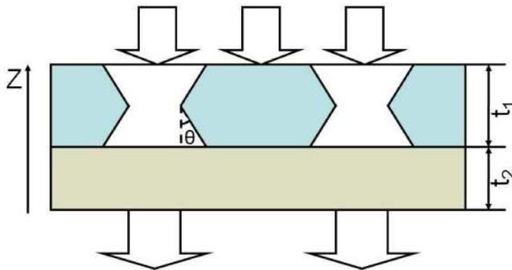
Fig. 1. The side view of the device structure. The thickness for the metallic layer is  $t_1$ , the thickness for the dielectric layer with a temperature dependent dielectric constant is  $t_2$ , and a circular CDC hole array with a semi-angle  $\theta$  will be made inside the metallic layer.
