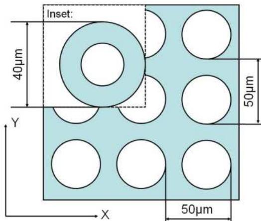
Fig. 2. The top view of the structure. The circular hole array is periodic in both the x and y directions, and the periodicity for the two directions are the same (50 $\mu\text{m}$ ). The inset shows the top view of a single circular hole.
