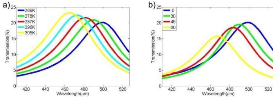
Fig. 4. Transmittance spectrum curves. (a) shows transmission spectrum with different temperatures. The converging angles are fixed at  $0^\circ$  (straight hole) for all cases. (b) shows transmission spectrum with different converging angles. The temperatures are fixed at 269 K for all cases.
