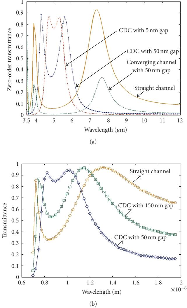
FIGURE 2: Zero-order transmittance for a normal incident plane wave on lamellar gratings in vacuum for different channel configurations, but with the same grating parameters as (a)  $d = 3.5 \mu\text{m}$ ,  $a = 0.5 \mu\text{m}$ , and  $t = 3.0 \mu\text{m}$  in gold film; (b)  $d = 650 \text{ nm}$ ,  $a = 300 \text{ nm}$ , and  $t = 500 \text{ nm}$  in silver film.
