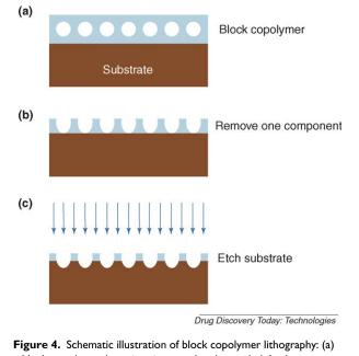
a block copolymer layer is spin-coated and annealed. It phaseseparates into close-packed periodic structures. (b) One component is selectively removed. (c) Pattern transfer through selective etching of the substrate material.
