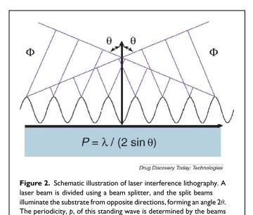
incident angles and the laser wavelength,  $\lambda$ ,  $p = \lambda/(2 \sin \theta)$ .
