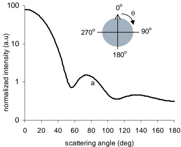
FIGURE 6. CALCULATED LASER INTENSITY DISTRIBUTION AROUND THE NANOSPHERE AS A FUNCTION OF SCATTERING ANGLE FOR AN INCIDENT LASER WAVELENGTH OF 1064 nm.
