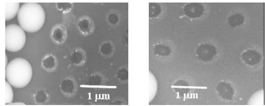
FIGURE 3. SEM MICROGRAPH OF HEXAGONALLY ARRANGED NANODENTS ON SILICON PRODUCED AT DIFFERENT LASER FLUENCES: (A) 4.0 mJ/Cm<sup>2</sup>, (B) 8.0 mJ/Cm<sup>2</sup>.
