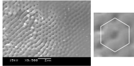
FIGURE 5. HEXAGONAL ARRANGEMENT OF NANOSTRUCTURES CREATED ON GLASS BY IRRADIATION WITH ND:YAG LASER.
