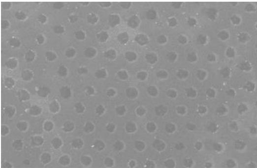
FIGURE 4. BOWL-LIKE NANO STRUCTURES CREATED ON HYDROGEN-TERMINATED SILICON SURFACE.
