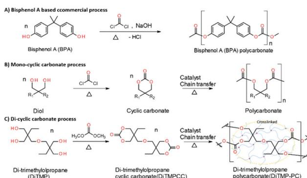
**Scheme 1** Polymerization pathways for the production of polycarbonates. (A) Commercial process from bisphenol A by reaction with phosgene. (B) Conventional process through mono-cyclic carbonate obtained by the reaction of diol and highly hazardous phosgene. (C) Green and sustainable process through a di-cyclic carbonate obtained by the reaction of polyol and dimethylcarbonate.
