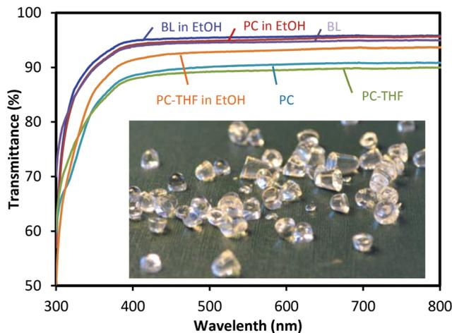
Fig. 4 Optical (transmittance) properties of the BPA-free PCs prepared from DTMPC (0.33 mmol) with 1.7  $\mu\text{mol}$  DBU and 35  $\mu\text{mol}$  1,3-PDO at 130 °C for 1 h. BL in EtOH; blank in ethanol, PC in EtOH; PC in ethanol, BL; blank, PC-THF in EtOH; PC (after submerging in THF for 15 min) in ethanol, PC; PC, PC-THF; PC after submerging in THF for 15 min. The inset shows the prepared PC pellets.
