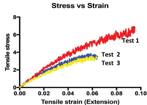
**Fig. 6** Tensile mechanical properties of BPA-free PC (PC-T) prepared from 0.33 mmol DTMP, 0.09  $\mu\text{mol}$  TBD and 14  $\mu\text{mol}$  1,3-PDO at 130 °C for 1 h.
