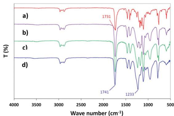
Fig. 3 FT-IR spectra of the reaction components and polycarbonate product formed during ROP of DTMPC at 130 °C. (a) DTMPC, (b) product in 15 min of ROP, (c) product in 30 min of ROP, and (d) product in 120 min of ROP.
