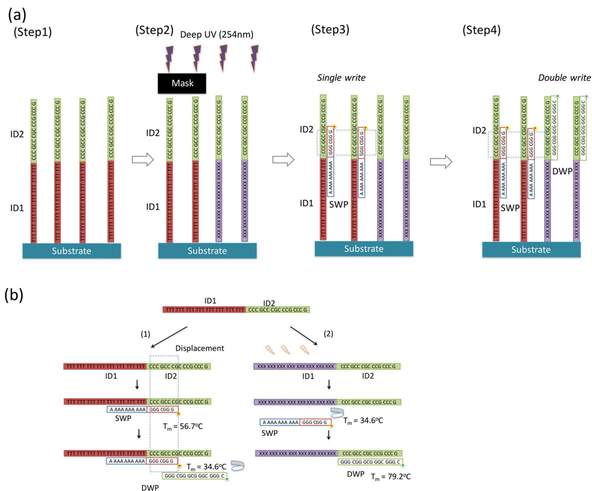
**Figure 2.** Scheme for the DNA double-write process. (a) Step 1, immobilization of the DNA double-write sequence (FWS:ID1&ID2) onto the glass substrate. Step 2, photomasking and UV exposure. Steps 3 and 4, hybridization of the red fluorescent SWP probe sequence 5'-Alex546-GGG CGG GAA AAA AAA AA-3' and the green fluorescent DWP probe sequence 5'-Alex488-GGG CGG GCG GGC GGG C-3'. (b) Effect of displacer and thymine dimer formation on probe hybridization and melting temperatures ( $T_m$ ).
