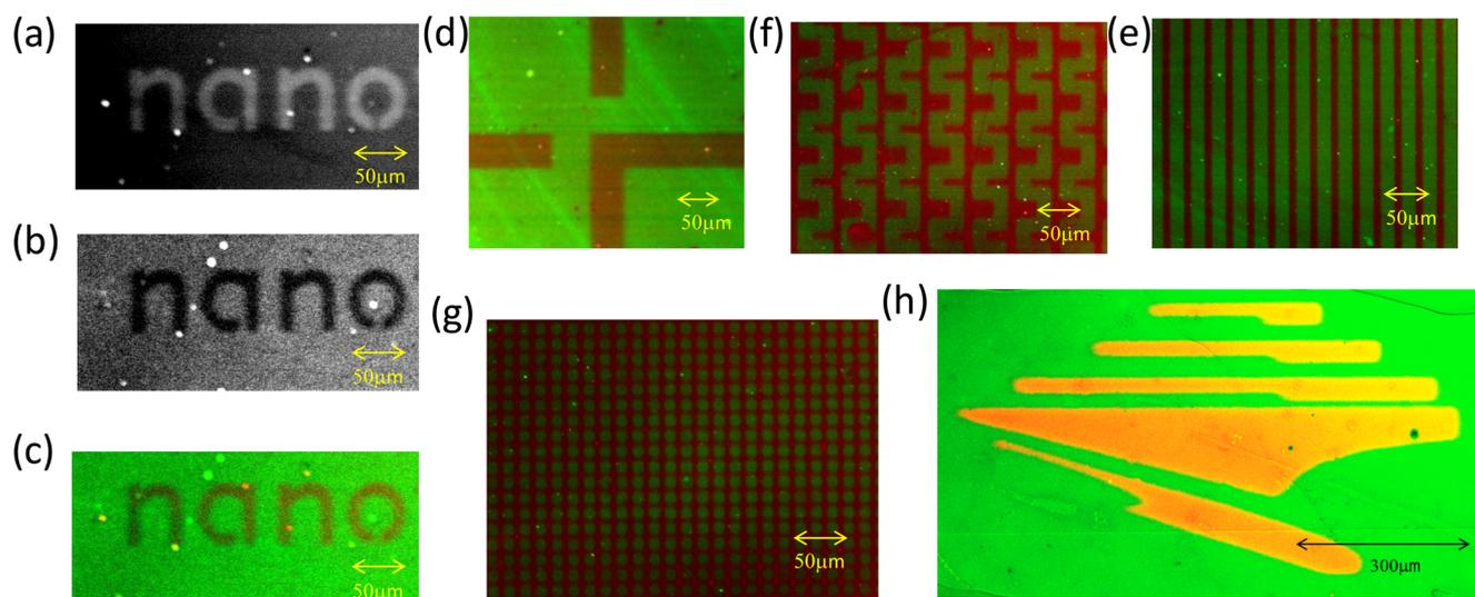
**Figure 3.** DNA double-write UV pattern images. (a) Black and white image of the single-write with red SWP probe hybridized on the letters. (b) Black and white image of the second write with DWP was hybridized in background. (c) False color image with single-write red SWP probe and second write green DWP probe. (d–h) More double-write images (first write color is red, second write color is green).
