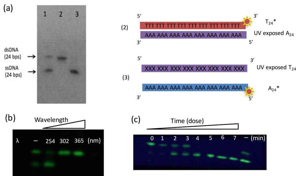
**Figure 1.** PAGE gels showing thymine dimer formation. (a) ds-DNA T<sub>24</sub>/A<sub>24</sub> and ss-DNA T<sub>24</sub> and A<sub>24</sub> lane 1, hybridized ds-DNA (T<sub>24</sub>\*IA<sub>24</sub>) when A<sub>24</sub> exposed to UV lane 2, dehybridized ss-DNA (T<sub>24</sub> and A<sub>24</sub>\*) when T<sub>24</sub> exposed to UV lane 3, (b) dehybridization of ds-DNA at different UV wavelengths, and (c) dehybridization of ds-DNA by UV dose.
