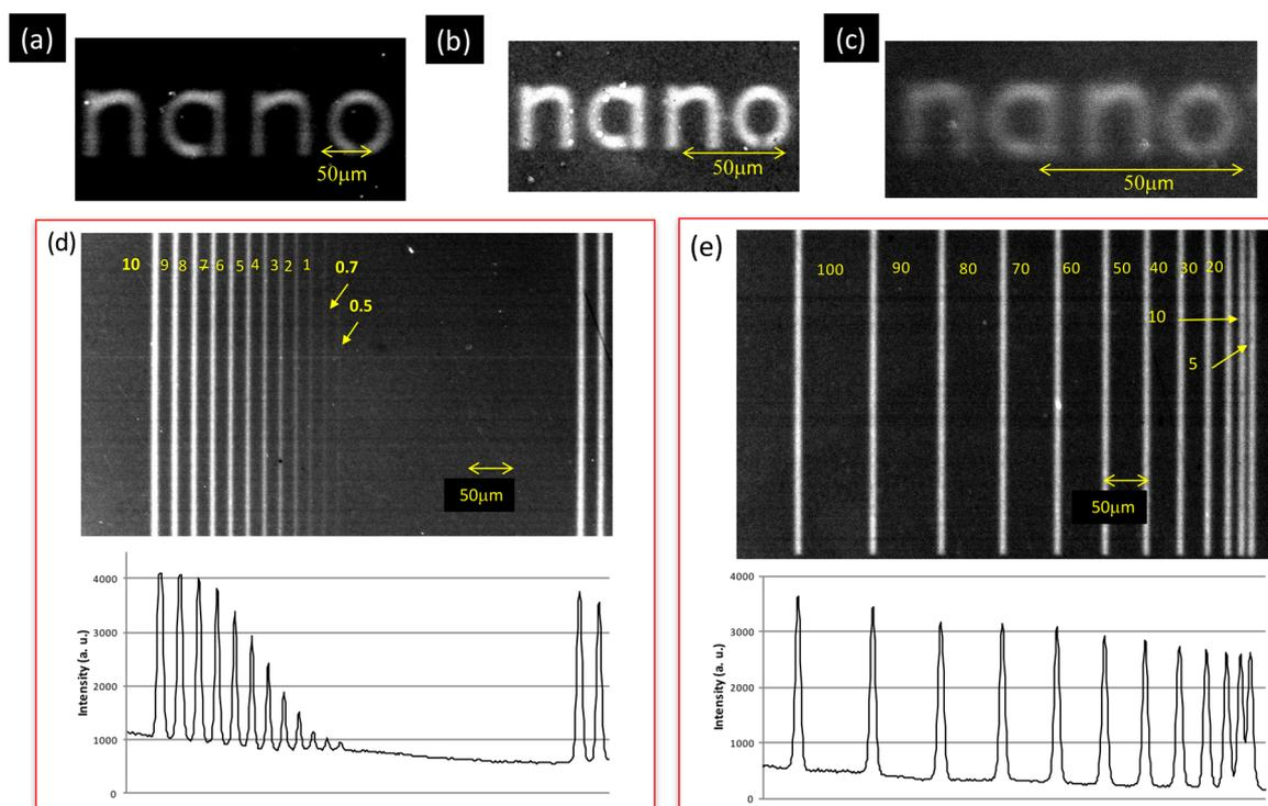
**Figure 4.** DNA double-write line widths with first level write. (a–c) Images of letters at 10  $\mu\text{m}$  line width, 5  $\mu\text{m}$  line width, and 2  $\mu\text{m}$  line width. (d) Line width resolution from 10  $\mu\text{m}$  to 500 nm. (e) Gap resolution from 100 to 5  $\mu\text{m}$ .
